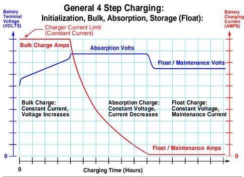
**Step 1) Initialization:** Red Light On or Red Light Flashing: Monitor Circuit verifies appropriate battery voltage levels and good electrical continuity between the battery and the charger DC output.
