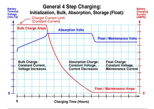
**Step 1) Initialization:** Yellow Light On or Yellow Light Flashing: Monitor Circuit verifies appropriate battery voltage levels and good electrical continuity between the battery and the charger DC output. **Step 2) Bulk Charge:** Yellow Light On, Green Light Off: Constant Current at Full Power. Bulk Charge ends at approximately 75% to 80% of full battery recharge.
